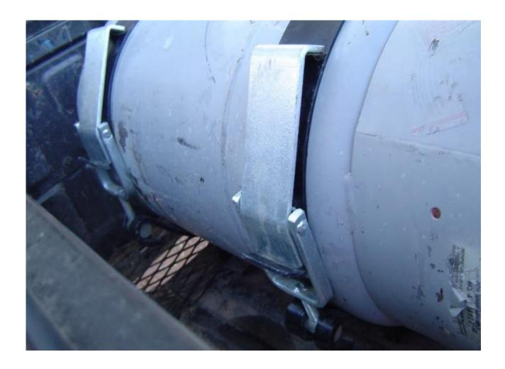
This is the correct installation of the tank brackets. They are adjustable by turning the hold downs. The brackets must be mounted to the truck with grade eight bolts and washers. You must also put big washers under the bottom of the truck to prevent the tank from pulling through the floor.
