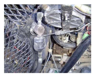
This is how the mixer and regulator look installed in the truck. The regulator needs to be mounted solidly. The hose in between is flexible. Be sure to check that all fittings have Teflon tape on them and are tight.
