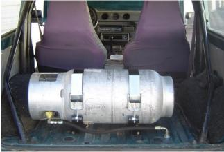
This is the bulkhead fitting back by the tank. It has a pressure relief device built into it. It is very important that all connections are tight and checked under pressure with soapy water. This is where the line connects in the back.
