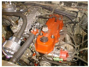
This is the mixer assembly bolted to the adapter. You will attach this to the throttle body. It will be a tight fit with the upper radiator hose and battery in the same area. We have found that aiming the air inlet downwards seems to fit pretty well. It is very important that there are no vacuum leaks from open ports on the intake manifold.
